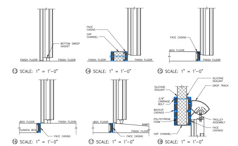
${\bf Page~4/4} \\ {\bf Bi-Parting~Horizontal~Manual~Slide~Door~with~Backup~Casings~and~Cap~Channels}$
